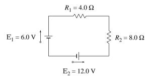
Find (a) the current in the circuit (including direction), (b) the power dissipated in each resistor, and (c) the energy transfer rate (including sign) at each battery.
