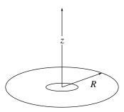
A washer (or annulus) with uniform surface charge density  $\sigma$  has outer radius R and inner radius R/5. What is the electric potential due to this charge at distance z above the center of the washer?
