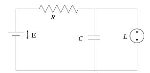
The lamp has these properties: When the voltage across it is less than the "breakdown voltage"  $V_L$ , the lamp has nearly infinite resistance. But when the voltage across the lamp reaches  $V_L$ , electrons are stripped from the lamp's gas atoms, creating a plasma with nearly zero resistance, and the lamp flashes.
