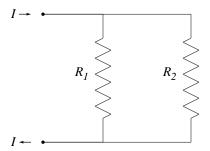
You know that the current I splits up so that i flows through  $R_1$  and (I - i) flows through  $R_2$  (Kirchhoff's junction rule). And you know that you can calculate i by demanding that the voltage drop across  $R_1$  is equal to the voltage drop across  $R_2$  (Kirchhoff's loop rule). This problem demonstrates a different method, the principle of minimum power dissipation, that can also be used to calculate the amount of splitting.
