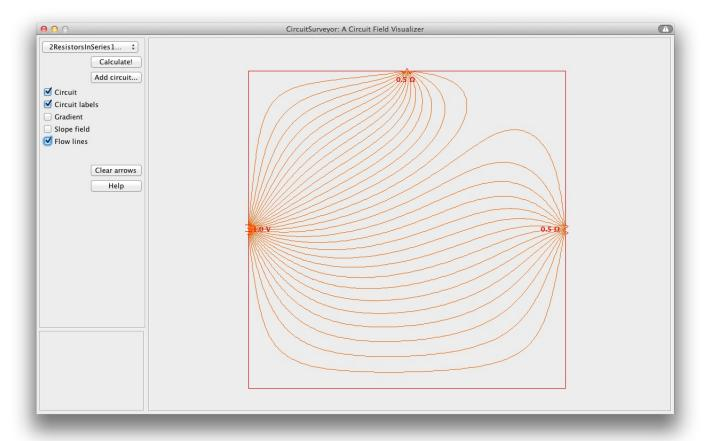
Figure 1: Poynting flow lines for a circuit with one  $1.0\,\mathrm{V}$  battery and two  $0.5\,\Omega$  resistors in series. The energy flows through space from the battery and arrives in equal amounts at each of the two resistors (15 flow lines each). (This is the circuit investigated in Ref. 4.)
