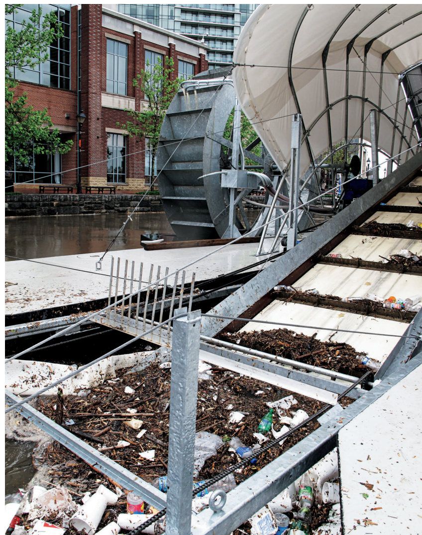
SUN SCREEN Solar panels power water pumps to turn the waterwheel. Right: The conveyor pulls the litter from the waterway.
